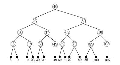
► Such a balanced binary search tree T on n points can be constructed in n log n time and it uses n storage.
