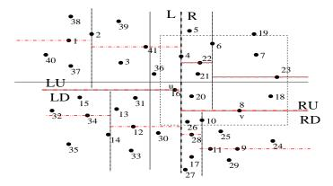
The set L (R) is split into two roughly equal sized subsets LU and LD (RU and RD), using point u (v) that has the median y-coordinate in the set L (R), and including u in LU (RU).
