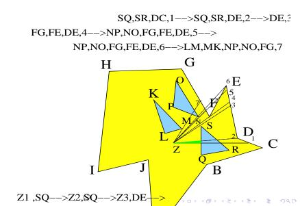
Computing the visible region in a polygon with opaque obstacles
