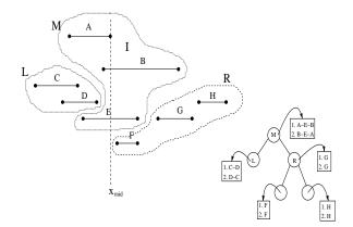
The set *M* has intervals intersecting the vertical line  $X = x_{mid}$ , where  $x_{mid}$  is the median of the x-coordinates of the 2*n* endpoints. The root node has intervals *M* sorted in two independent orders (i) by right end points (B-E-A), and (ii) left end points (A-E-B).
