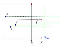
Use an interval tree of all the horizontal segments and the right bounding edge of the query rectangle like X or X'.
