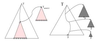
$T_{assoc(v)}$  is a binary search tree on y-coordinates for points in the leaf nodes of the subtree tooted at v in the tree T.
