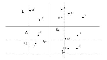
Using two 1-d range queries, one along each axis, solves the 2-d range query.
