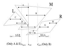
For  $x_{query} < x_{mid}$ , we do not traverse subtree for subset R. For  $x'_{query} > x_{mid}$ , we do not traverse subtree for subset L. Clearly, the cost of reporting the k intervals is  $O(\log n + k)$ . REPORTING (PORTIONS OF) ALL RECTILINEAR SEGMENTS INSIDE A QUERY RECTANGLE
