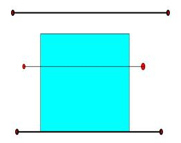
Report all (horizontal) segments that cut across the query rectangle or include an entire (top/bottom) bounding edge. Use either the right (or left) edge, and the top (or bottom) edge of the query rectangle.
