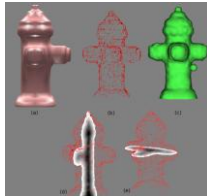
(a) A .obj model of a water hydrant (courtesy 'www.turbosquid.com') (b) The sampled sparse point set after preprocessing, (c) zero-isosurface points of the reconstructed object, (d) the distance field for a vertical cross-section of the reconstructed object, and (e) the same for a horizontal cross-section.
