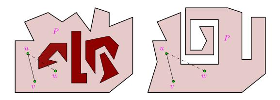
A polygon P is defined as a closed region in the plane bounded by a finite set of line segments (called *edges* of P) such that there exists a path between any two points of P which does not intersect any edge of P.
