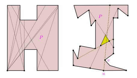
The polygonal region of P is decomposed into convex components where every component is bounded by segments that contains any two vertices of the polygon.
