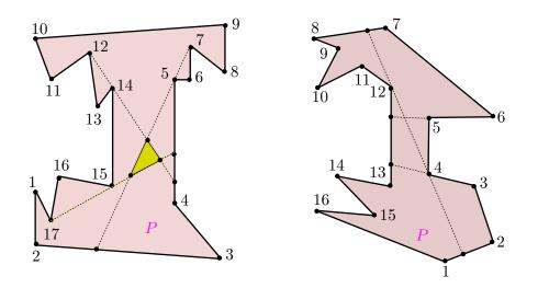
Vertices 7, 12 and 17 together can see the entire boundary of the polygon but the shaded region is not visible from any of these vertices.
