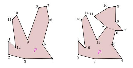
A simple polygon is called a *fan* if there exists a vertex that is visible from all points in the interior of the polygon.
