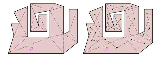
**Lemma:** Every triangulation of a simple polygon P of n vertices uses n - 3 diagonals and has n - 2 triangles.
